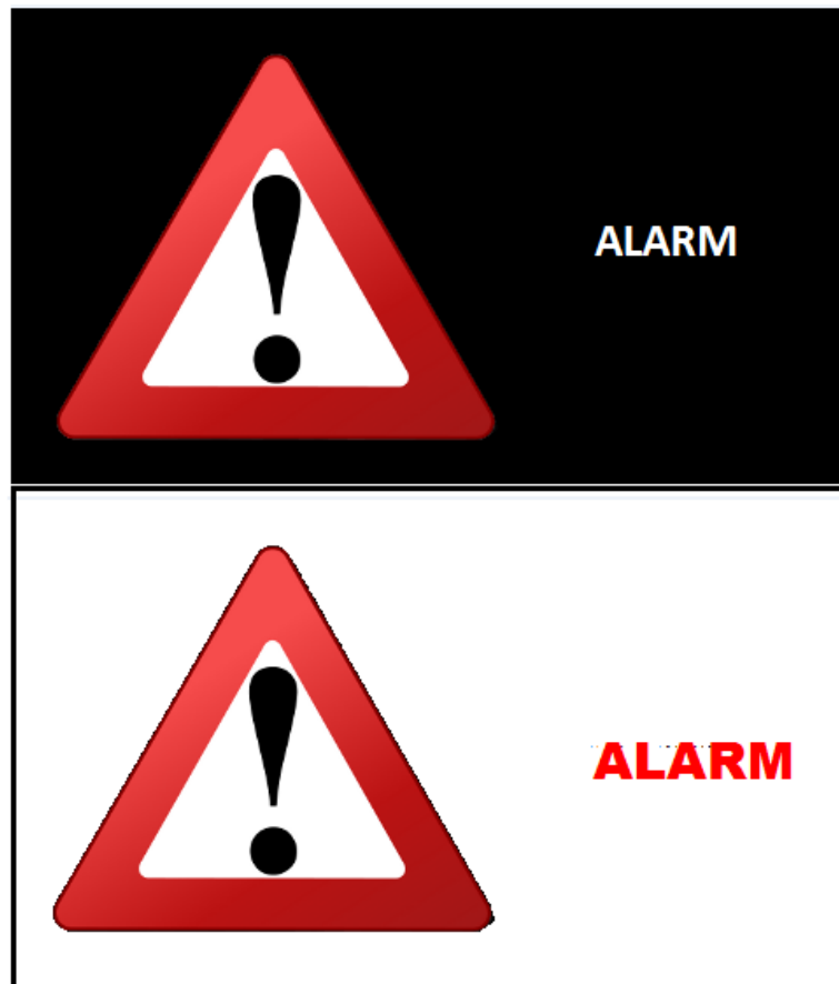
Alternating visual display of ALARM Condition
